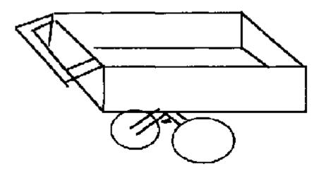
This type of cart has a payload of 2-3 cubic meters, is frequently made of wood, can have bicycle wheels or other small vehicle wheels, and the axle is usually metal, as is the handle. Some sort of metal frame workaround the base of the cart holds it together and makes it more sturdy.
