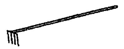
4. The heaps of wastes are levelled by a three-tine drag (or rake) with a handle about 2 metres long and the flanks are formed to an angle of about 45°. Levels and strip width are guided by pegs driven earlier.
