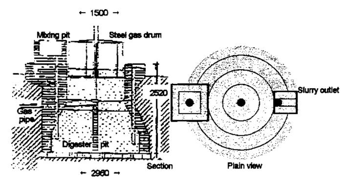
Taper design of steel drum biogas plant
