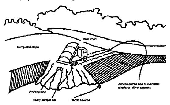
Strip width 6 metres; only one vehicle at a time on working face; capacity 30-40 tonnes/day.
