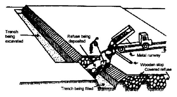
The trench method of controlled tipping. The heaps of refuse ale levelled and famed to a 45° slope using a long - handled rake, and covered by at least 150 mm of soil excavated from the next bench. The width of the trenches should not be less than their depth.
